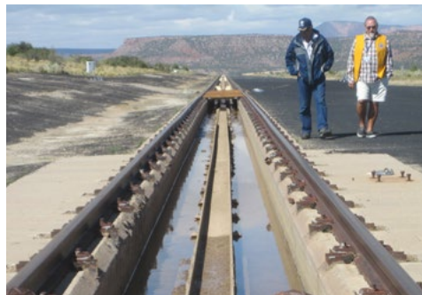
Tracks from the Hurricane Mesa Test Facility. Each single-piece track is 12,000 feet long to accelerate rocket sleds up to Mach 1.
